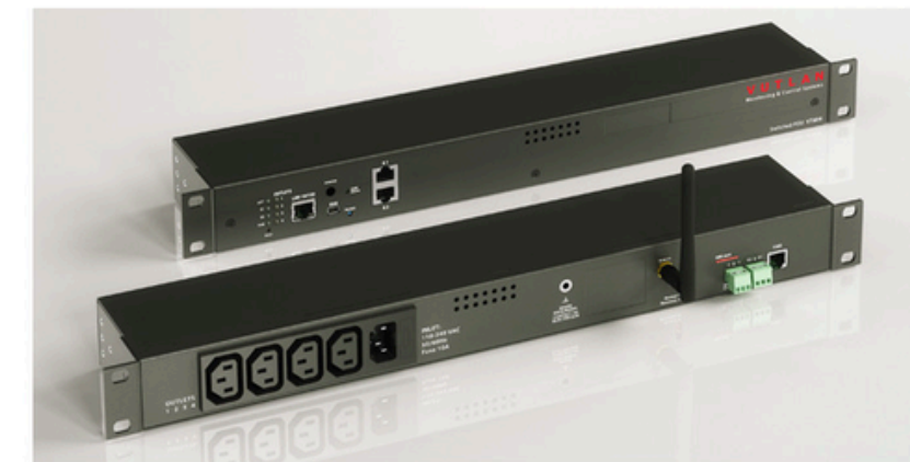
"VT604 / Switched PDU" + "VT700 / GSM modem" VT700 is ordered separately. Terminal plugs are included in the delivery.
